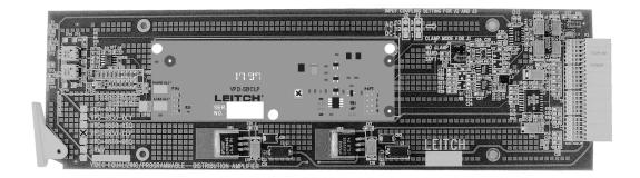
Figure 8-2. VPD-6830-CLP Video Equalizing DA with Hard and Soft White Clip.
